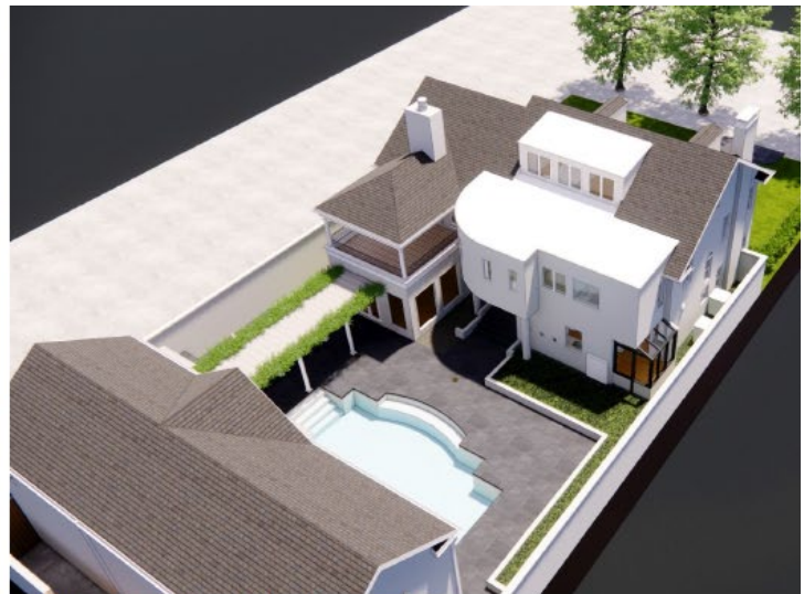
RENDERING OF PROPOSED LEVEL 2 ADDITION TO REAR OF MAIN HOUSE. NEW ROOF DORMER ADDED TO LEVEL 2.5, WITH MEMBRANE ROOFING TO MATCH 1980s ADDITIONS. NEITHER OF THE ADDITIONS WOULD BE VISIBLE FROM NORTH BLVD.
