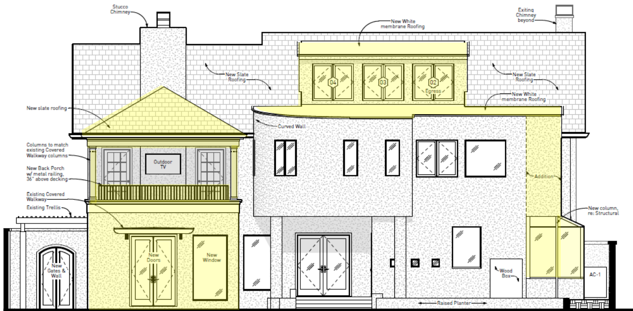
03 Exterior Elevation - North, View from Backyard Scale: 3/16" = 1'-0"
